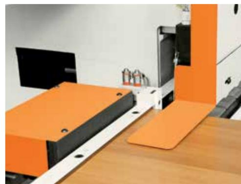
The pre-arrangement and the bar code reader allows a quick reading of the working program. Available on request.
