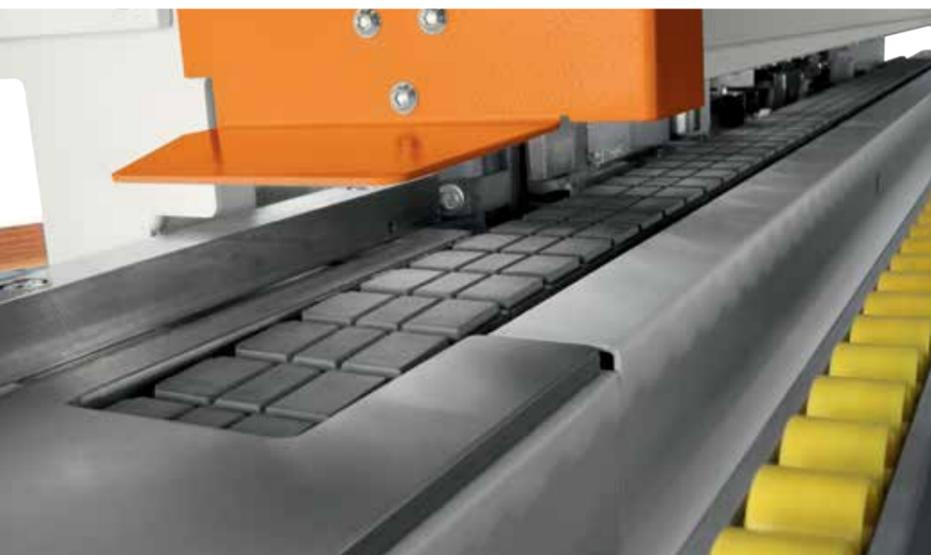
Linear and perfect feed thanks to feeding chain track with high grip rubber coated pads and sliding on industrial chain. High resistance to lateral loads thanks to special guides with one circular section and one flat section.
